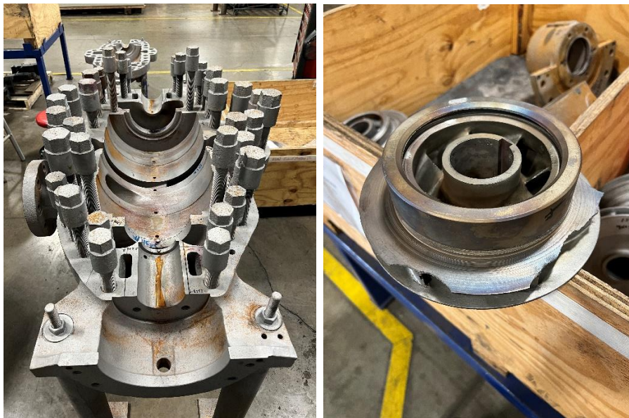
Image 2 + 3: The pump in question was a between-bearing, six-stage type working with propylene carbonate, with damage to all the stationary and rotating elements contained within
