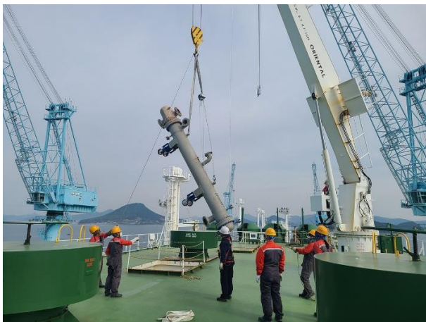
Image 3: Compressor gas cooler tube being removed for service
