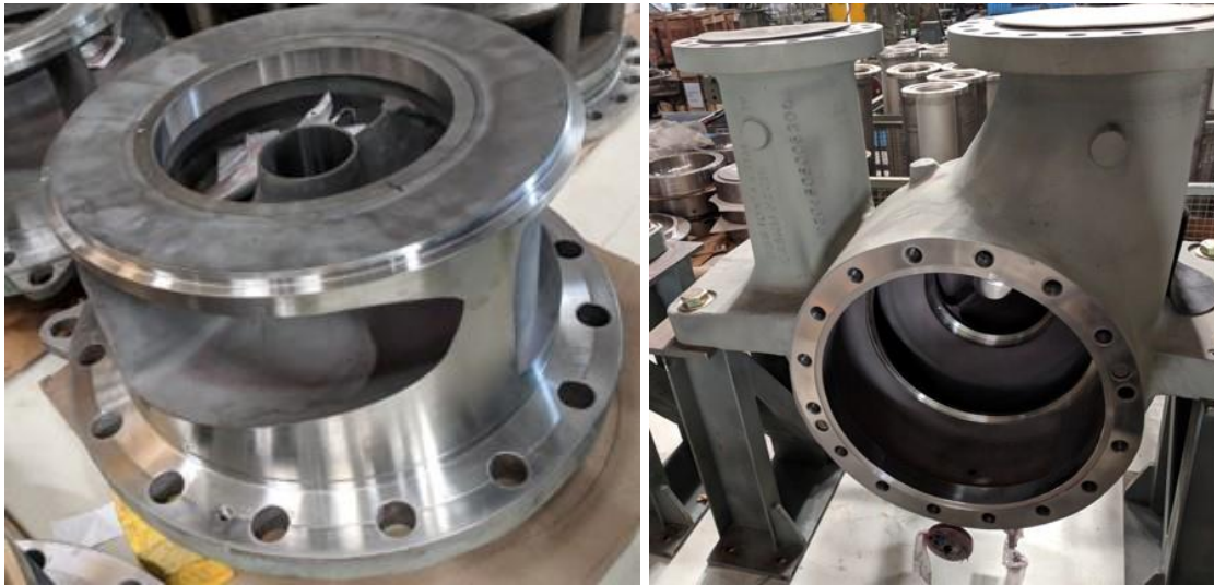
Image 3 + 4: Material upgrades using high-chromium steel.
