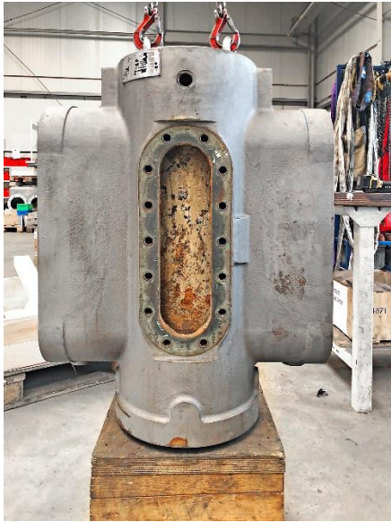
Image 1: The cylinder before it was repaired at Burckhardt Compression Germany's Service Center.
