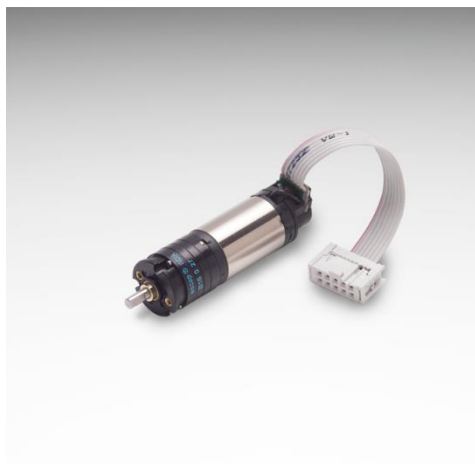
Image 3: Portescap's MR2 magneto-resistive encoder helped to achieve accurate position control for the robotic joints
