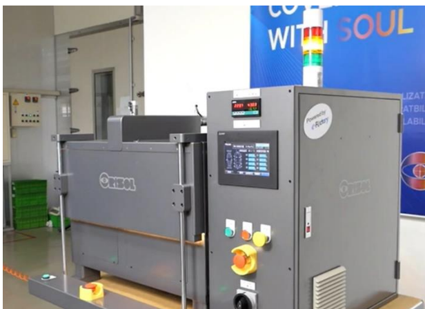
Image 2: Orisol saw its OFA240 series upper to sole flash activator machine as an ideal candidate to benefit from the principles of TSN technology. (© Orisol)
