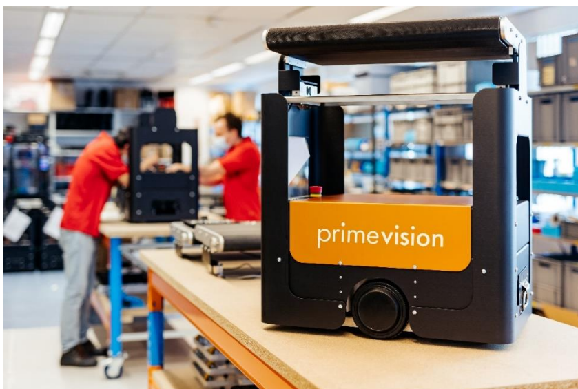
Image 4: Prime Vision's robotic systems can carry parcels from 100 g to 35 kg
