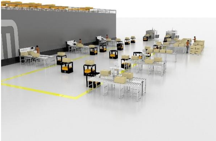
Image 3: Robots can be programmed to travel new routes over and over again, and the number of them can be scaled up and down
