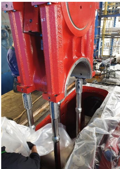
Image 2: Replacement of bearings and overhaul of connecting rod.
