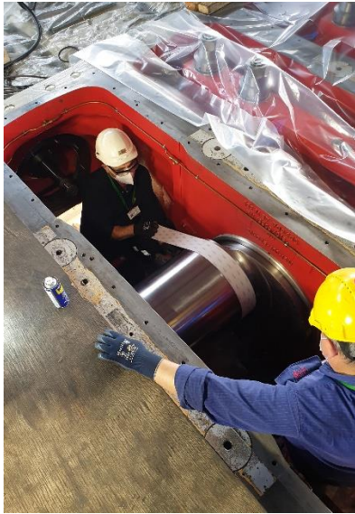
Image 1: Overhauling the crank gear and realigning the crankcase.
