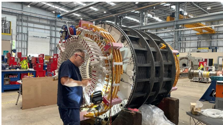
Image 4: Changes to the winding would need to be carried out while preserving the Ex certification of the units.
