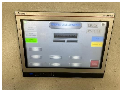
Image 3: An intuitive and user-friendly GT2510 widescreen HMI maximises process visibility and accessibility, helping operators monitor and interact with the drives, identify anomalies and interpret alarms.
