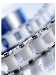
**Image 1:** Tsubaki's BS PC chain offers the benefit of a stainless base, with link plates manufactured from SUS304 and spring clips from SUS301. These materials combine with inner chain links of engineering plastic to produce high levels of corrosion resistance.
