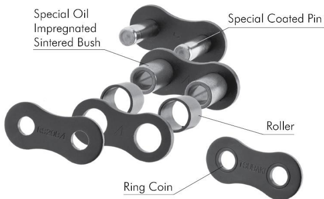
Image 2: The lube-free technology of the Lambda Chain includes bushes that are sintered, meaning the material is formed into a solid mass through heating without liquification.
