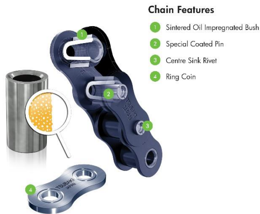
Image 1: The lube-free technology of the Lambda Chain includes bushes that are sintered, meaning the material is formed into a solid mass through heating without liquification.
