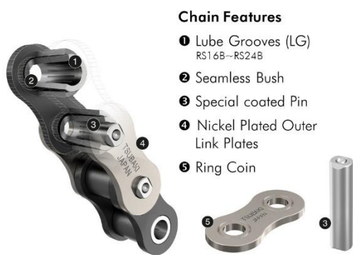
Image 2: The Titan chain's pins have a hard coated, low friction surface for increased wear and corrosion resistance. The seamless bushes also include Lube Grooves that hold the oil between the pin and the bush, the point of greatest contact, maintaining lubricati
