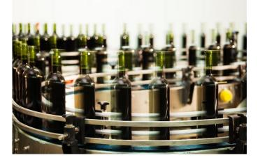
**Image 1:** A German wine producer uses a series of conveyors to transport their bottles through the production process. At the end of the system, the bottles are buffered and accumulated on a spiral conveyor. (Image Source: istock-97151143 – mrfotos)
