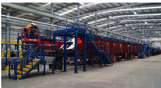
Image 3: The jigs provided by KM Tools allow the main subassemblies to be held in position for welding and finishing
