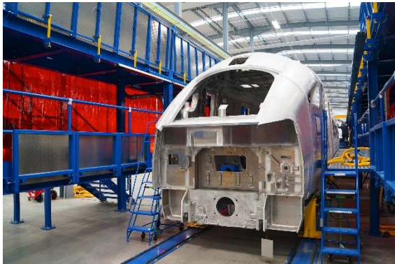
Image 4: The jigs provided by KM Tools allow the main subassemblies to be held in position for welding and finishing
