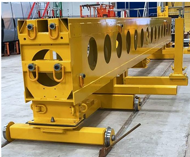
Image 4: Alstom uses KM Tools SmartLine Jigs for construction of trains for new Cairo Monorail
