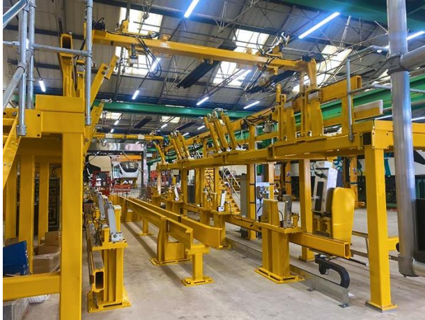
Image 1: Alstom uses KM Tools SmartLine Jigs for construction of trains for new Cairo Monorail
