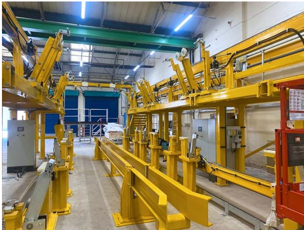
Image 3: Alstom uses KM Tools SmartLine Jigs for construction of trains for new Cairo Monorail
