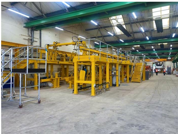
Image 2: Alstom uses KM Tools SmartLine Jigs for construction of trains for new Cairo Monorail
