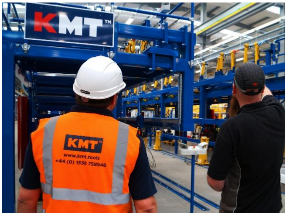
Image 2: The SmartLine jigs produced by KMT for this project are entirely bespoke, designed to accommodate specific train models manufactured by Hitachi Rail.
