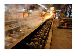
**Image 1:** Bauer Gear Motor has completed a three-year retrofit project for the roller table conveyor drives at Aperam's Châtelet facility in Belgium.
