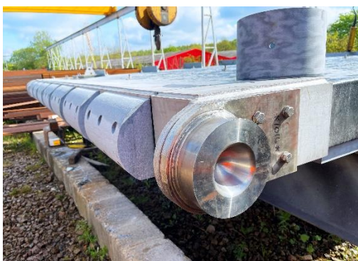
Image 5: All steel components below the water line were manufactured in stainless steel
