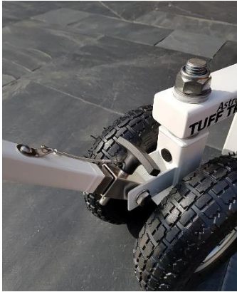
Image 4: WDS detent pins are used to lock the handle into place.
