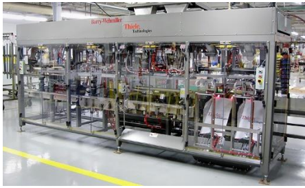
Image 1: Tolomatic's electric screw actuators increase the flexibility of bag size handling
