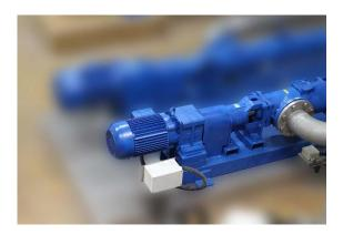
**Image 2:** With the PMSMs installed, the pumps consumed 24% less energy when pumping primarily sludge compared to using an IE3 asynchronous motor.
