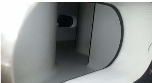
Image 3: Cylinder water chamber after cleaning
