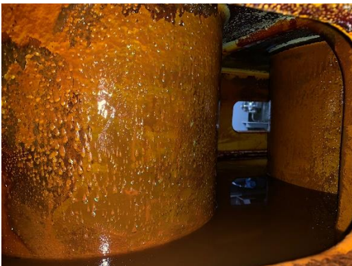
Image 2: Corrosion caused to cylinder water chamber due to an incorrect glycol mixture
