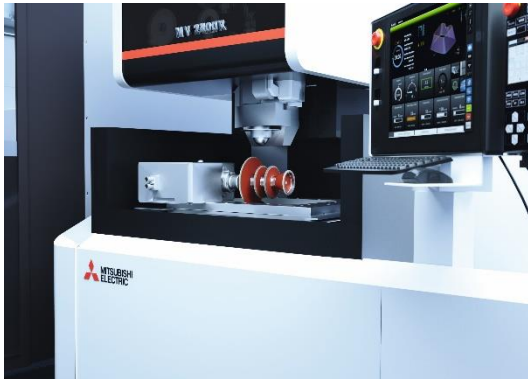
Image 1: EDM-DRESS – the perfect technology for an improved grinding process, using a multi-purpose high-precision wire cut EDM system. [Source: Mitsubishi Electric Europe B.V.]
