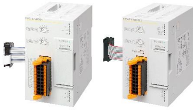
Image 1: Two new safety modules for Mitsubishi Electric's compact PLCs form the basis of an integrated safety system. [Source: Mitsubishi Electric Europe B.V.]
