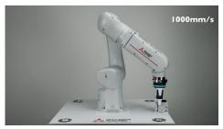
**Image 1:** To further maximise the return on investment the MELFA ASSISTA cobot offers a high-speed operation mode for when it is not working alongside humans – meaning it can be used as a standard industrial robot as well. [Source: Mitsubishi Electric Europe B.V.]
