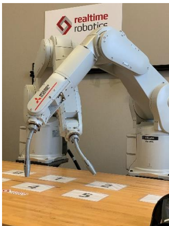
Image 2: Mitsubishi Electric industrial robots with Realtime Robotics' technology embedded can work safely and collision-free in an unstructured and dynamic environment. [Source: Mitsubishi Electric Europe B.V.]
