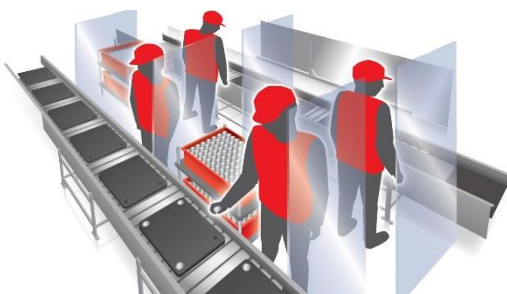
Image 3: Some plant managers are considering using screens between workers, but this is not a panacea as there can be operational limitations [Source: Mitsubishi Electric Corporation, Japan]
