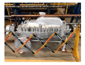
**Image 1:** Sulzer Indonesia carried out detailed inspections of the units and conducted a full refurbishment of the pumps, bringing them back to as-new standard.
