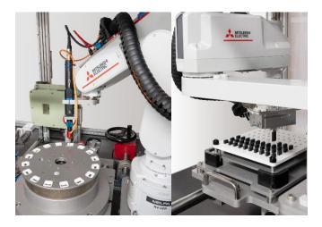
**Image 2 + 3:** To overcome the challenge of the magnets becoming brittle after being magnetised, Horizon chose two selections from Mitsubishi, their four-axis RH-6CH and six-axis RV-2FR robots
